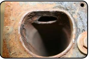
Install the busings into the cross member tube. The flat part of the busing needs to align with the flat part of the cross member tube. Use grease and a dead blow hammer to install the bushing.
