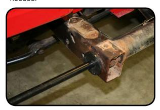
Install the spacers on both sides of the torsion bar. If needed use a chisel and hammer to open up the relief cut to install the spacer onto the shaft.
