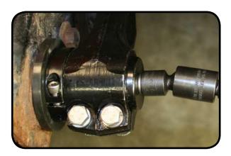
10. Torque the sway bar arm pinch bolts to 50 Ftlbs using a 9/16" socket and wrench.
