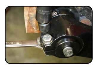
11. Tighten the spacer bolts using a 3/16" allen.
