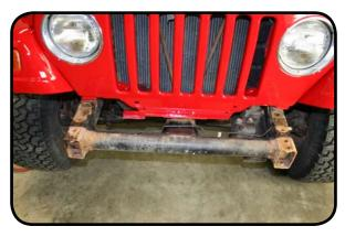
4. Check the cross member tube for any obstructions. Clean the tube using a barrel sander.
