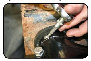
Install the sway bar links on the outside of the sway bar arm, and on the inside of the axle mount. Use blue tread locker on the sway bar arm bolt.
