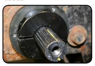
8. Install the sway bar arms onto the torsion bar. It is critical that both of the arms are on the same spline. (Use reference marks to aid in the install.) Make sure the torsion bar is about 1/4" inward on both sway bar arms.
