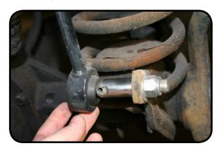
3. Remove the bolts from the sway bar mount using a 15mm socket or wrench. (Use tape to protect the paint.)
