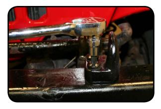
Remove sway bar links at the axle using an 18 mm socket (if using quick disconnects just slide them off the mount pin) Remove the pin or factory bolt.
