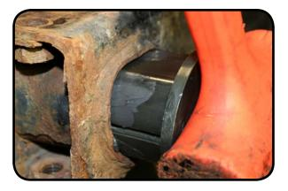
Grease the inside of the bushing and install the torsion bar. Use a dead blow hammer if needed.
