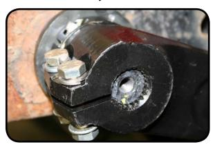
9. Install the end caps using 9/16" socket and blue tread locker. Torque to 20 Ft-lbs.
