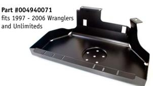
**Note:** If you don't have a body lift, you will need to install one prior to installing the HD gas tank skid plate, or you will have to use the TeraFlex spacer kit P/N 004970400, sold separately. With a body lift, you can push the HD skid all the way up against the frame and enjoy the additional ground clearance.
