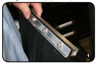
Place mud flap onto the mounting bar and install locking nuts on the back. Make sure that you do a left and a right. (Photo #2)
