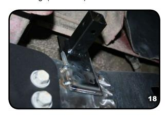
17. Once brackets are welded in place paint the welded area to protect from rust and corrosion. (Photo #19)
