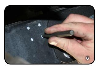
6. Drill out four holes with a 17/64 drill bit.(Photo #7,8)
