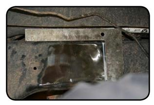
5. Measure 2 1/2" forward from the rear scribe line. Mark and use a square to mark the area that will be removed.
