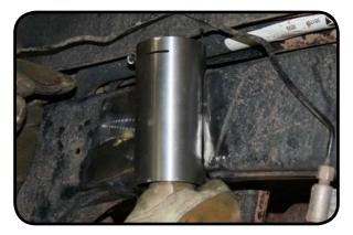
10. Place speedbump mount in the frame so the bottom of the mount is 1/8" below the frame and tack it into place.
