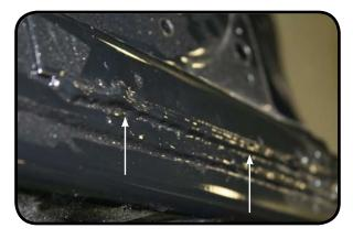
7. Using a cut off wheel cut in from the scribe lines at a 45 degree angle.
