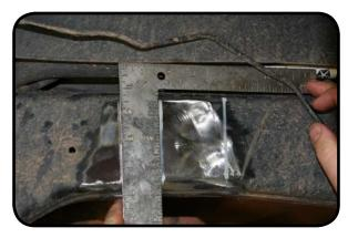
6. The depth of the cut needs to be 1 1/8" on the top and bottom of the frame. This should put the new speedbump mount flush with the coil bucket weld on the top of the frame.(Use the arrows below for reference. View from the top of the frame.)
