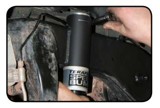
15. Install the new bumpstop pads on the axle using the supplied hardware.
