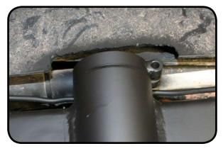
14. Install the TeraFlex speedbump into the new mount. Use silicon on the speedbump and slide it up into the mount. Use the supplied bolt to tighten the pinch clamp.
