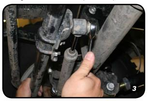
8. Loosen the tie rod ends and drag link end at the knuckle and hit the face of the knuckle to loosen the taper and remove the tie rod and drag link ends. (Photo #4)
