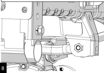
Loosely install the lower inside 9/16" x 1" bolt. Use a lock washer under the bolt head. To start the nut, tape the nut to the 7/8" end wrench as shown and slide it down between the frame and cross member support bracket. Repeat for other side.
