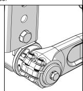
Using a small arbor press or vise, press the misalignment spacers into the rubber bushings of each sway bar link. Grease the inner diameter of the bushings and the outer diameter of the spacer to aid in installation.
