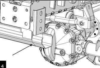
Later model JKs will require cutting the cross member support as shown. Use a square to mark a cut line 4 5/8" down.
