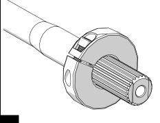
Tap a wedge (cold chisel or large flat screw driver) into the pinch clamp relief on the forged sway bar arm. Make sure the chisel doesn't protrude into the splines.
