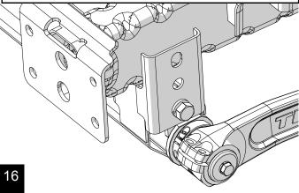
Torque the outer bolt to 55 ft-lbs while using an alignment tool (such as a large punch). Remove the alignment tool
