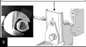
Tap the torsion bar bushings into the frame brackets.
