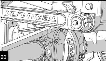
Install the four (Grade 8) 3/8" x 1 1/2" long pinch bolts in the arms. Don't forget the lock washers and blue thread locking compound. Alternate tightening the bolts on the arms to equalize the load between the bolts. Final torque all pinch bolts to 50 ft-lbs. Torque the alignment spacer cap screws to 8 ft-lbs.
