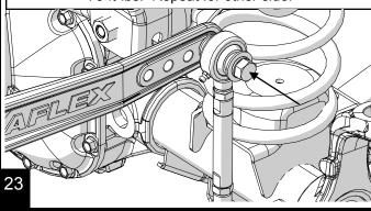
Install the lower link using the included 1/2"-13 bolts and stover nuts. Apply blue thread locking compound to the bolts and torque to 75 ft-lbs. Repeat for other side.
