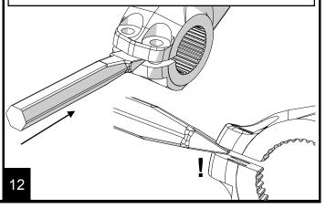
Orient the forged sway bar arm as shown before tapping the arm onto the dual splined bushing/torsion bar assembly.
