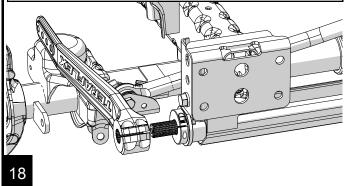
Tap the forged arm onto the torsion bar until there is approximately 1/4" between the end of the bar and face of the forged arm. Remove chisel.
