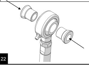
Orient the sway bar link as shown for easy zerk access. Choose your desired sway bar rate hole and install the upper link using the included 1/2"-20 bolt. Apply blue thread locking compound and torque bolt to 75 ft-lbs. Repeat for other side.
