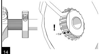
Apply blue thread locking compound to the 3/8" x 3/4" long stainless steel bolt and install the sway bar end cap along with the lock washer. Only snug the bolt, do not torque yet.
