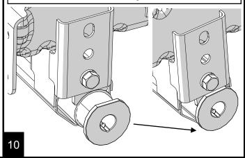
Loosely install the included 1/4"-20 allen cap screw, position the collar as shown and slide it onto the torsion bar.
