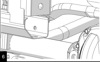
Insert left and right frame brackets. The lower hole will be further forward, with each hole lining up with a factory hole
