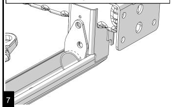
Loosely install the 9/16" x 1" bolt, don't forget the lock washer. Repeat for other side.
