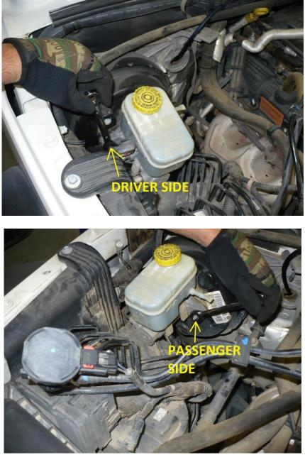
5) Install the 4018-RHD bracket using the factory nuts removed in step 4.
