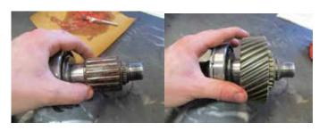
Note: Clean the packing oil out of the oiling hole of the low range output gear. Bearing damage will result if oiling hole filled with packing oil.
