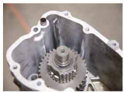
**STEP 31**Area to clearance for counter shaft gear.
