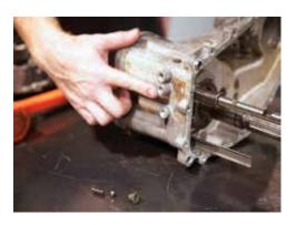
Insert the bushing locking ball into shaft, secure
