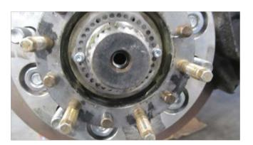
**STEP 8**Install new thrust washer
