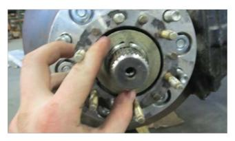
**STEP 10**Install TG spindle washer
