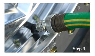
Connect the garden hose to the adapter and turn the water on. Water will start flowing into the tire. Periodically turn the water off and then push in the valve button. If the water level is above the valve core, then water will come out of the button. If air comes out, then the water level is below the valve core. Once the desired water level has been reached, remove the water fill adapter and reinstall the valve core.
