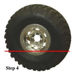
To prevent damage to your air pressure gauge, we recommend that you check your tire pressure only when the valve core is above the water line.
