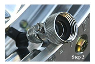
Next, thread the water fill valve onto the valve stem. Note that the push button valve on the side of the fill valve should be accessible.
