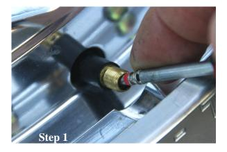
Start by removing the valve core and allow all of the air to escape from the tire.
