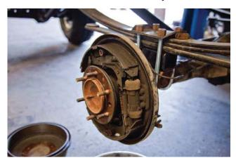
**STEP 4 - REMOVE BEARING POCKET NUTS**
